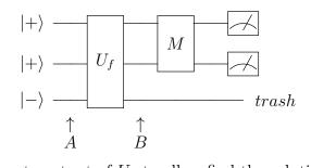
M is a circuit that converts output of  $U_f$  to allow find the solution by measuring. We are not going to discuss how it's implemented here since this is not directly related to phase kickback.
